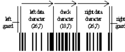
Figure 5.6.1.3 - 2 GS1 DataBar Limited Bar Code Structure
