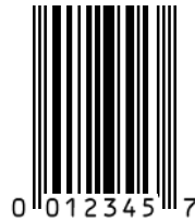
Figure 5.2.1.3.4 - 1 UPC-E Bar Code (Encoding 00123400057 by Zero-Suppression)
