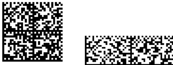
Figure 5.6.3.2-3. Segmented GS1 DataMatrix symbols: Square and rectangular formats (sizes of these GS1 DataMatrix symbols are larger than what would be used in a typical application so that typical alignment patterns can be easily seen.)
