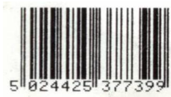
Figure 5.9.5.12-1. Symbol with edge determination problem
